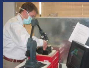
Figure 4. Freehand cutting navigated with a Microscribe G2X arm.
