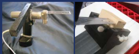
Figure 1. The MiniBIRD sensor was mounted away from the saw (left), and a plastic vice was used (right) to minimize interference.
