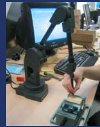
Figure 3. Digitizing with a Microscribe G2X.
