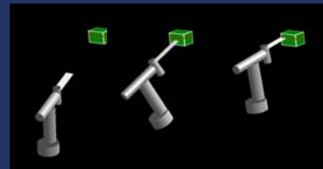
Figure 2. The saw image moves in real time on the computer screen as the surgeon cuts the block.
